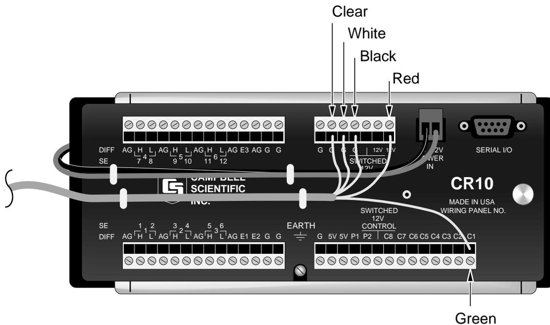
FIGURE 2. SR50 Wiring for CR10(X) SDI-12 Example
