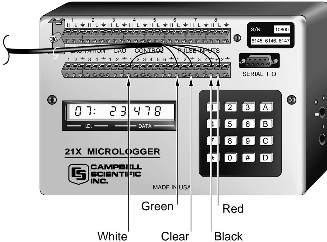
FIGURE 4. SR50 Wiring for 21X Pulse Example
