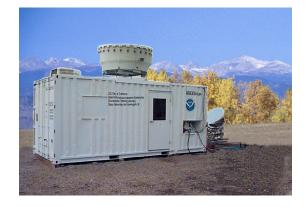
*Figure 1. Photo of the MMCR Package showing* the radar antenna (roof) and MWR reflector (right side).
