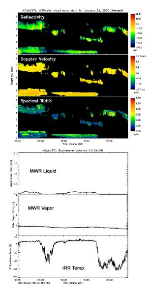
Figure 2. An example of MMCR-Package data for a 24-h period with high, middle, and low clouds. The upper three panels are time-height displays of Doppler moments from the radar; the lower three panels are time series plots from the radiometers.
