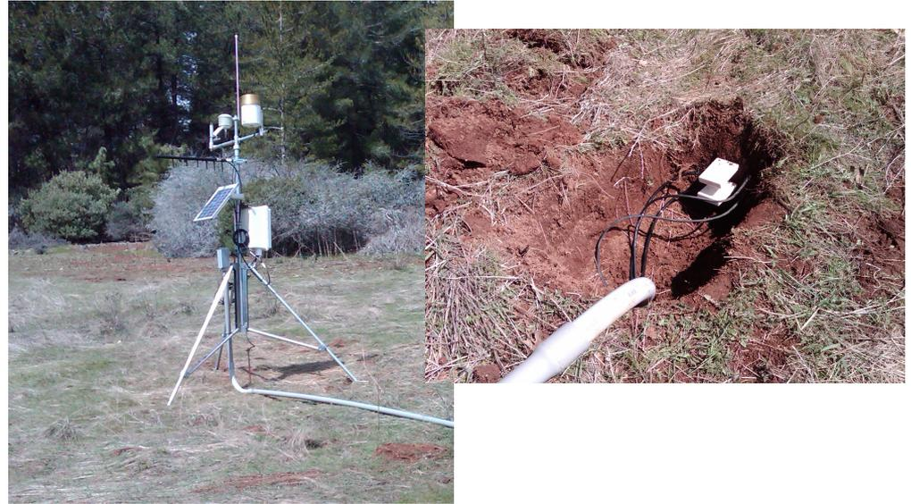
A typical setup for one of HMT's surface sites with a tripod and solar panel/battery for instrument power. The site measures temperature, relative humidity, rainfall, soil temperature, and soil moisture at two levels (10 and 15 cm). Data are transferred to our data processing hub by internet cel modems and shared with the AQPI system.
